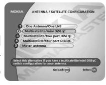
For each LNB you connect to the DiSEqC switch, the following configuration has to be performed.
